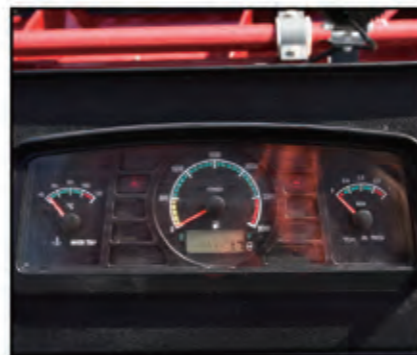
The instrument panel is concise and clear, showing the machine condition
